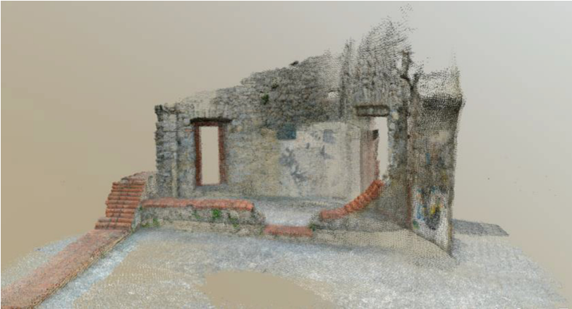
Fig. 3. 3D model reconstructed using RTAB-Map [18]
