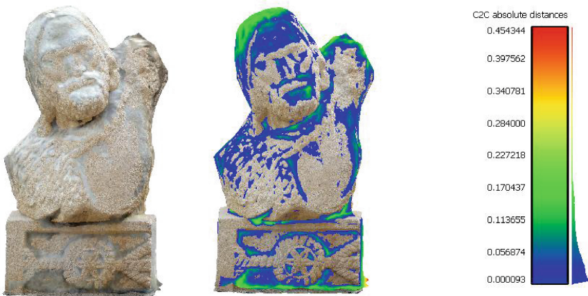
Fig. 9. Aligned point cloud (a) Photogrammetry/Tango models absolute distances (b)
