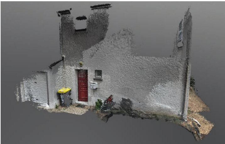
Fig. 4. 3D model reconstructed using Matterport Scenes [25]
