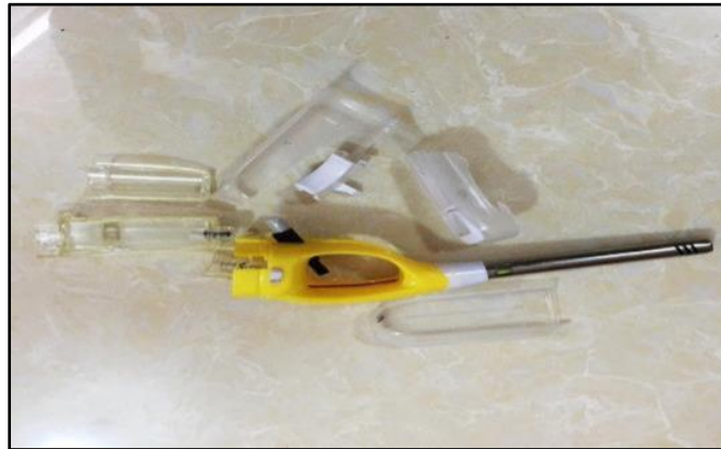
Figure 3. Gas lighter exploded.
