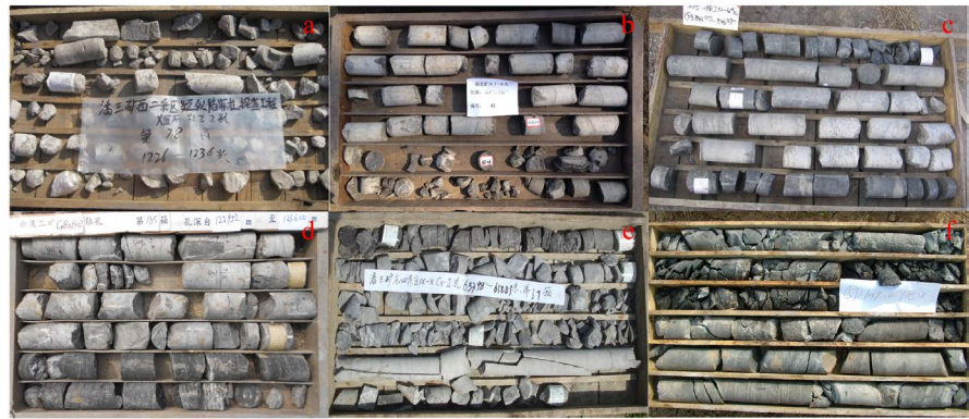
Figure 1. Taiyuan group limestone core graphs. (a) graben-horst combination structure; (b) horst; (c) graben; (d) strike-slip fault; (e) imbricate thrust structure; (f) other structure.
