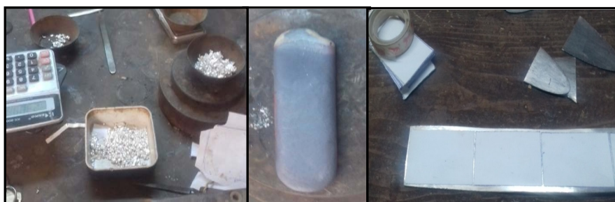
Figure 1. Manufacturing to silver coupons: (a) Pure silver pieces; (b) Shape of resulting rod after casting; (c) Cutting coupons after ductility and hammering processes.
