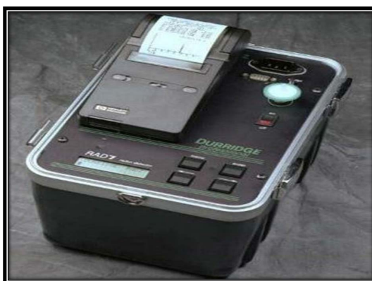
Figure 1. The durrIDGE RAD-7 electronic continuous radon monitor with an HP printer mounted for immediate printing of results.
