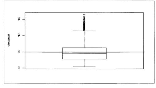
Figure 8: Box plot for wind speeds at 30 metres height at site B
