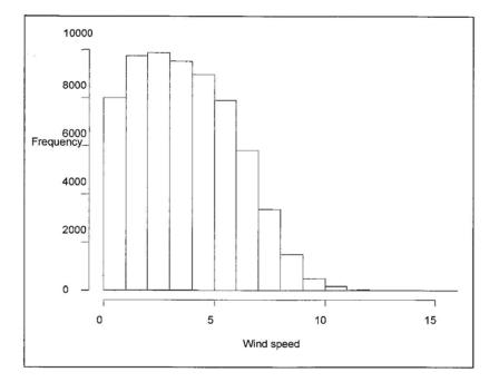
Figure 2: Frequency distribution of wind speed at site A at 20 metre height
