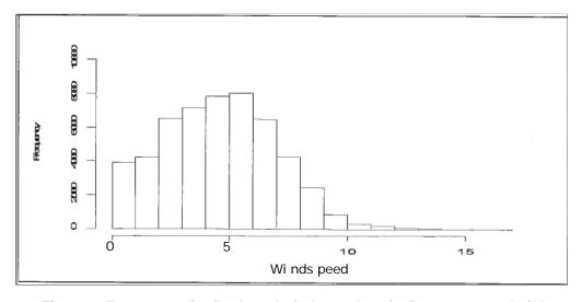
Figure 7: Frequency distribution of wind speed at site B at 30 metres height
