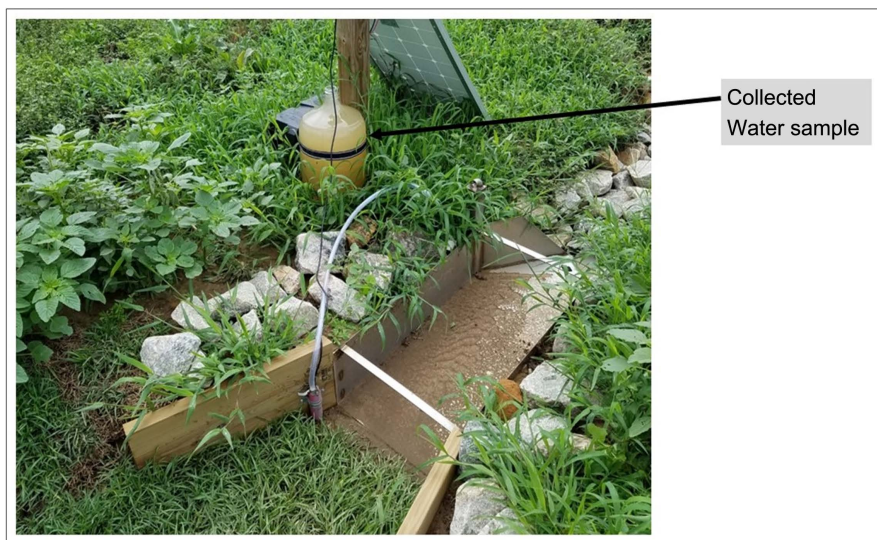
Figure 16. A composite water sample is collected from a H-flume during a runoff event.
