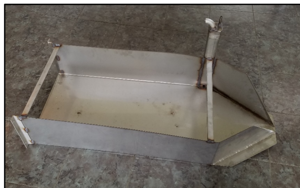
Figure 5. A completed stainless steel H-Flume ready for installation in the field site.
