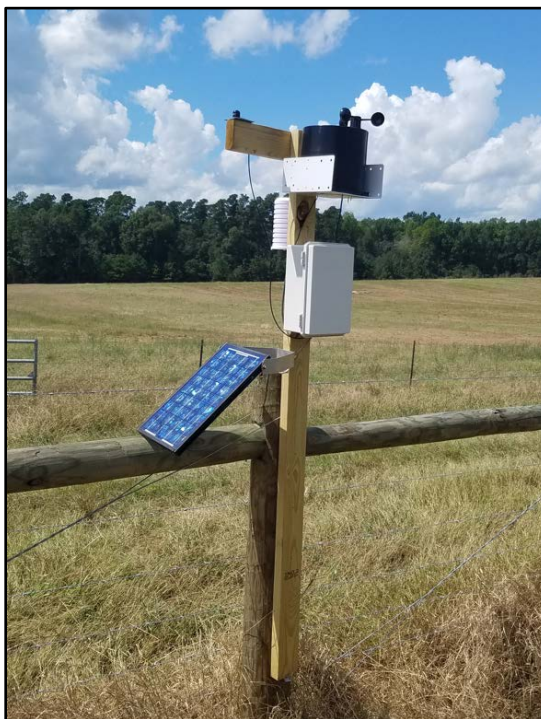
Figure 12. The IoT weather station located near the field site.
