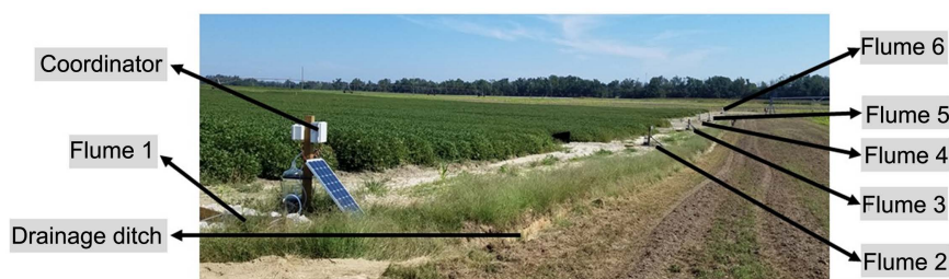
Figure 10. The layout of the coordinator and nearby end nodes (flumes) positions in the field.
