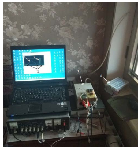
Figure 3. First prototype of ArtAr-HDF during solar microwave emission measurements in light clouds sky during sunset in Yerevan 9 January, 2020. 1—Light cloudy sky, 2—The sun during sunset (the maximum is \sim 160 K), 3—Gray Body with an emissivity of \sim 0.95 at +2^\circ\text{C} (the mean is \sim 261 K), 4—First prototype of ArtAr-HDF, 5—Third prototype of ArtAr-HDF.
