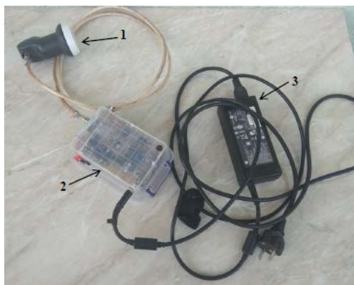
Figure 19. ArtAr-HDF. 1—LNB, 2—A low-frequency part, 3—A power supply.
