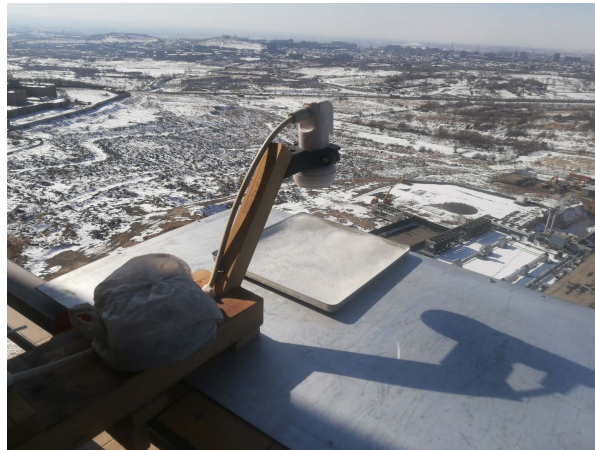
Figure 10. An experiment with a duralumin tray with frozen thin (8 mm) ice layer on a duralumin sheet.
