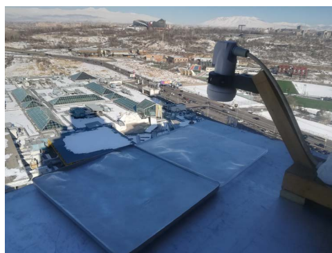
Figure 13. An experiment with two 8 mm thin ice layers on a duralumin sheet.
