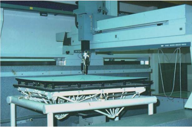
**Figure 2. The support frame with two panels of the Millimeter Radio Telescope’s surface in coordinate measuring machines. The measurement accuracy was  $<5 \mu\text{m}$ , and the average panel surface error was  $27 \mu\text{m}$ .**
