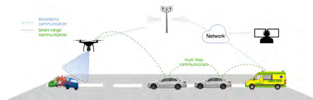
FIGURE 26. A UAV is used as a flying RSU that broadcasts a warning about road hazards that have been detected in an area not pre-equipped with an RSU (Flying Roadside Units) [169].
