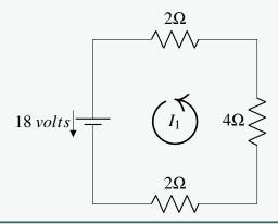
**Solution.** Begin in the bottom left corner, and trace the circuit in the counter clockwise direction. At the first resistor, multiplying resistance and current gives  $2I_1$ . Continuing in this way through all three resistors gives  $2I_1 + 4I_1 + 2I_1$ . This must equal the voltage source in the same direction. Notice that the direction of the voltage source matches the counter clockwise direction specified, so the voltage is positive.
