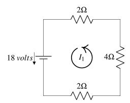
In the above figure, the current  $I_1$  has been labelled with an arrow in the counter clockwise direction. This is an entirely arbitrary decision and we could have chosen to label the current in the clockwise direction. With our choice of direction here, we define a positive current to flow in the counter clockwise direction and a negative current to flow in the clockwise direction.
