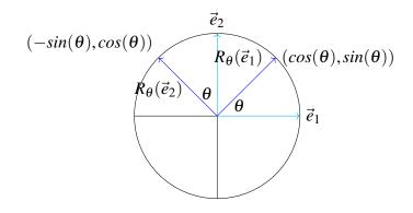
From Theorem 5.6, we need to find  $R_{\theta}(\vec{e}_1)$  and  $R_{\theta}(\vec{e}_2)$ , and use these as the columns of the matrix A of T. We can use cos, sin of the angle  $\theta$  to find the coordinates of  $R_{\theta}(\vec{e}_1)$  as shown in the above picture. The coordinates of  $R_{\theta}(\vec{e}_2)$  also follow from trigonometry. Thus
