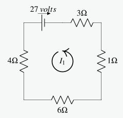
**Solution.** Begin in the top left corner this time, and trace the circuit in the counter clockwise direction. At the first resistor, multiplying resistance and current gives  $4I_1$ . Continuing in this way through the four resistors gives  $4I_1 + 6I_1 + 1I_1 + 3I_1$ . This must equal the voltage source in the same direction. Notice that the direction of the voltage source is opposite to the counter clockwise direction, so the voltage is negative.
