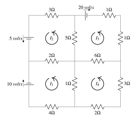
The current in amps in the four circuits is denoted by  $I_1, I_2, I_3, I_4$  and it is understood that the motion is in the counter clockwise direction. If  $I_k$  ends up being negative, then it just means the current flows in the clockwise direction.
