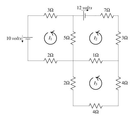
The current in amps in the four circuits is denoted by  $I_1, I_2, I_3$  and it is understood that the motion is in the counter clockwise direction. If  $I_k$  ends up being negative, then it just means the current flows in the clockwise direction.
