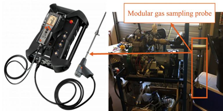
Figure 10. Illustration of the Testo 350 with the probe connected to the exhaust DE.
