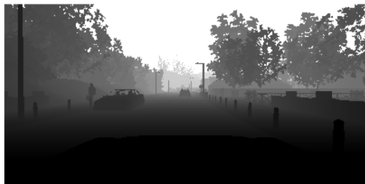
FIGURE 10. A depth image produced from synthetic lidar data, generated in the CARLA [164] simulator.
