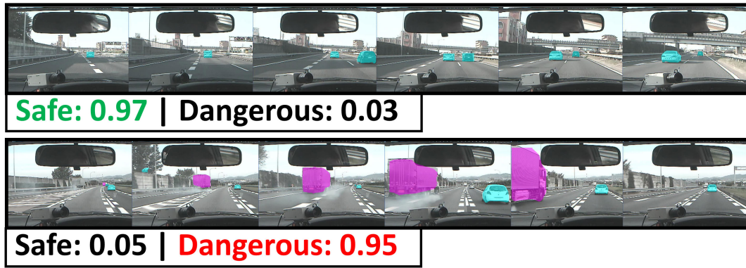
FIGURE 14. Assessing the overall risk level of driving scenes. We employed an open-source 1 deep spatiotemporal video-based risk detection framework [211] to assess the image sequences shown in this figure.
